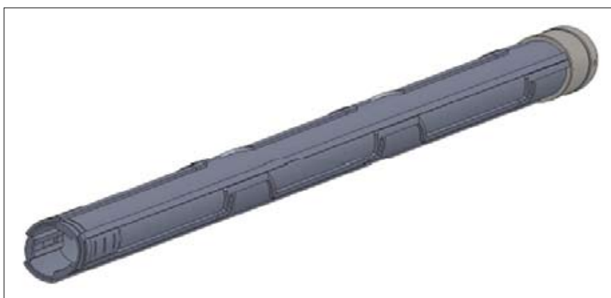
Kelly's solid model made by CAD 3D parametric Assigned material with mechanical and physical properties
