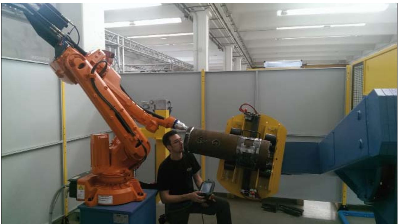
Welding robot for Kelly bar terminals
