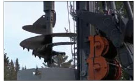
Conical Rock Auger OD 2,6 m - SHD type
