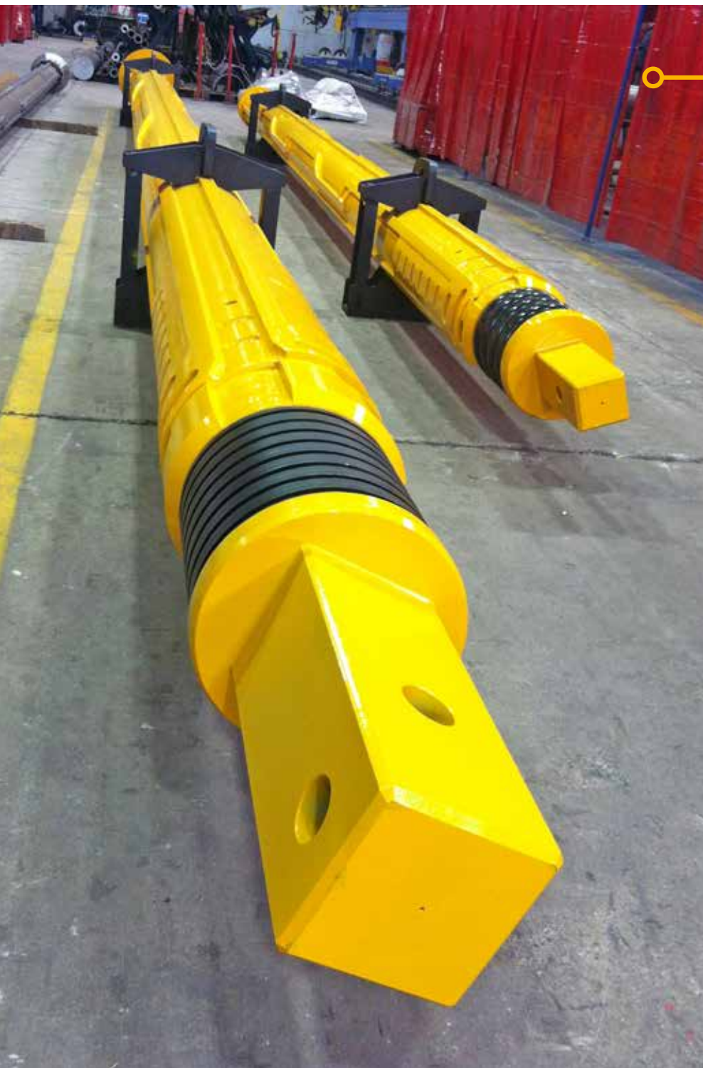
Interlock kelly bars to drill up 60 m (on the left side) and 36 m (on the right side)
