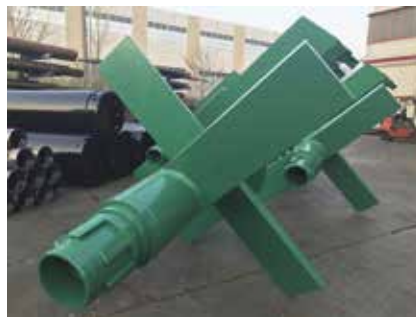
> Detail of the upper joint used to connect the tip with the bars
