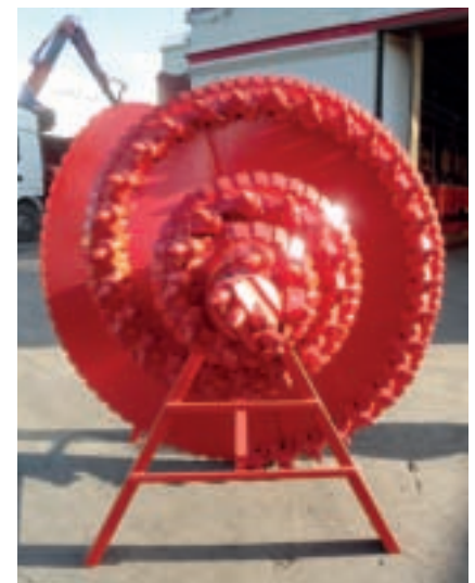
The geometry of the chisels arrangement is optimized for reaching excellent cutting performance.
