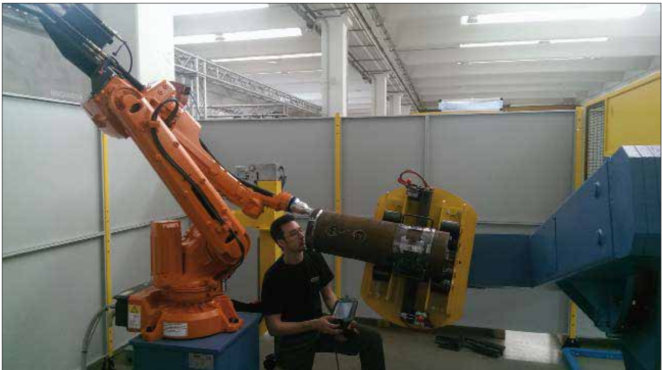
Welding robot for Kelly bar terminals
