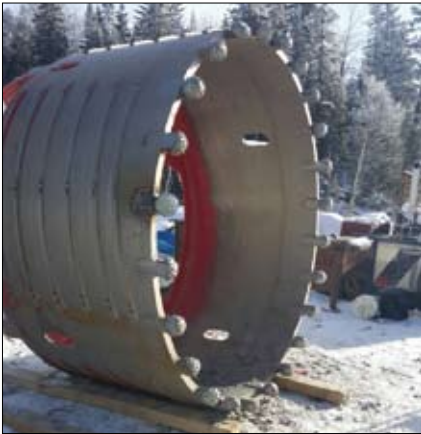
Core barrel with Roller Bits OD 2.6 m - SHD type
