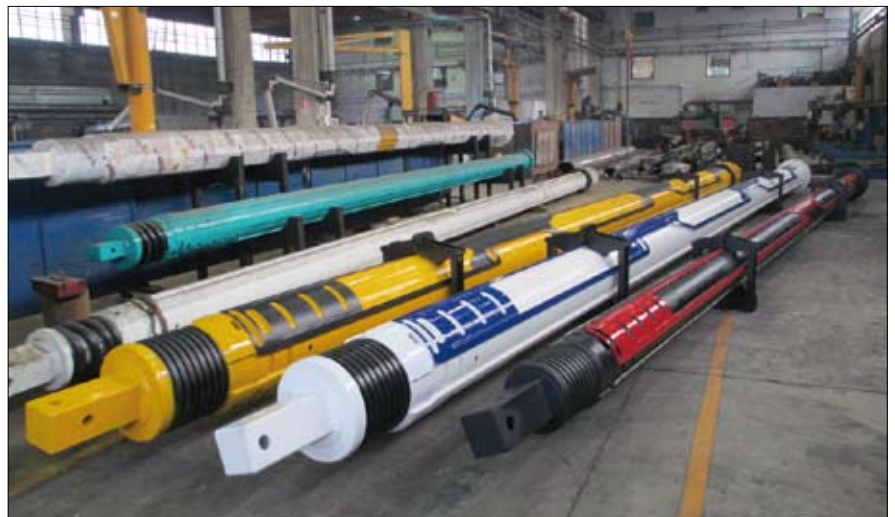
Kelly bar for piling rigs with torque between 200 and 390 kNm, 160 and 320 kNm and 140 and 460 kNm
