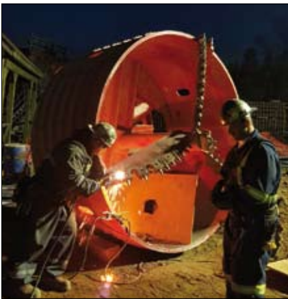
Chisels replacement on Core Barrel Cross Cutter OD 2.6 m - SHD type
