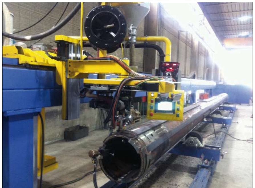
Automated process of submerged arc welding of Kelly bars
