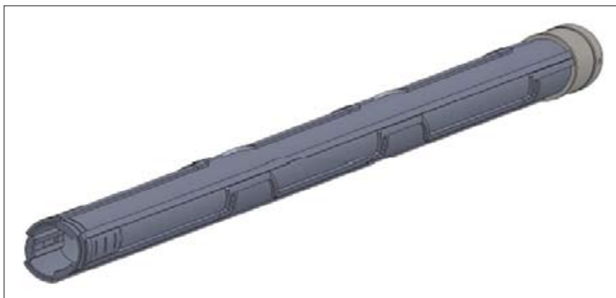
Kelly's solid model made by CAD 3D parametric Assigned material with mechanical and physical properties
