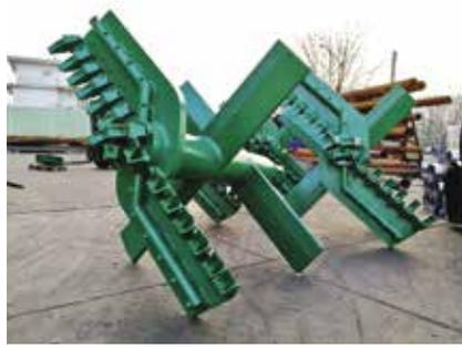
> Soil mixing Tip OD 3000 mm
