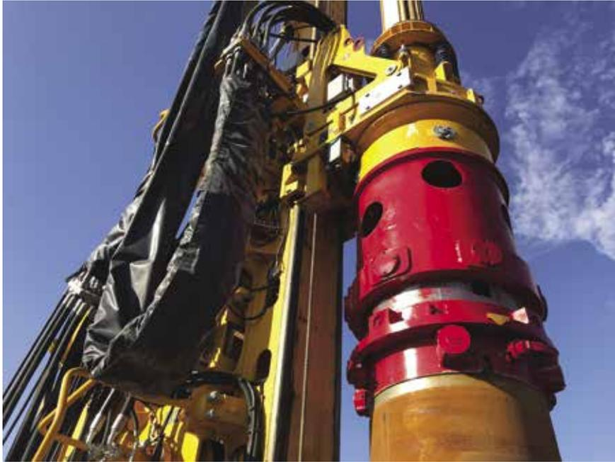
➤ Automatic Casing Drive Adaptor OD 880/800 mm
