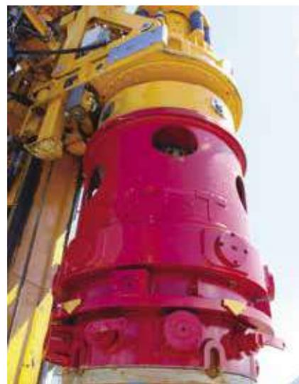
► The operator is able to dis/connect the casing column to the Auto CDA without any other personnel help, so they can directly manage the work from the piling rig cabin
