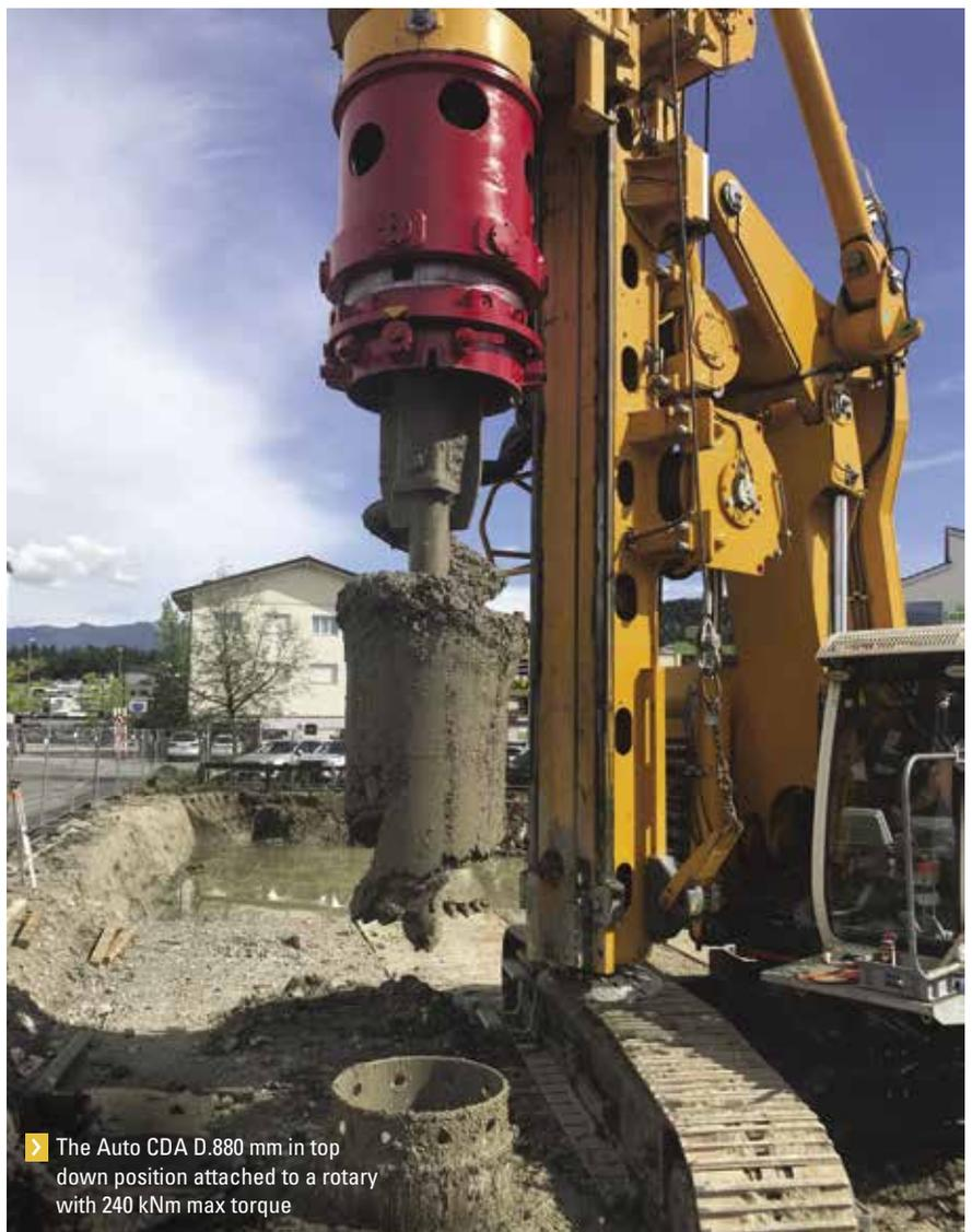
➤ The Auto CDA D.880 mm in top down position attached to a rotary with 240 kNm max torque
