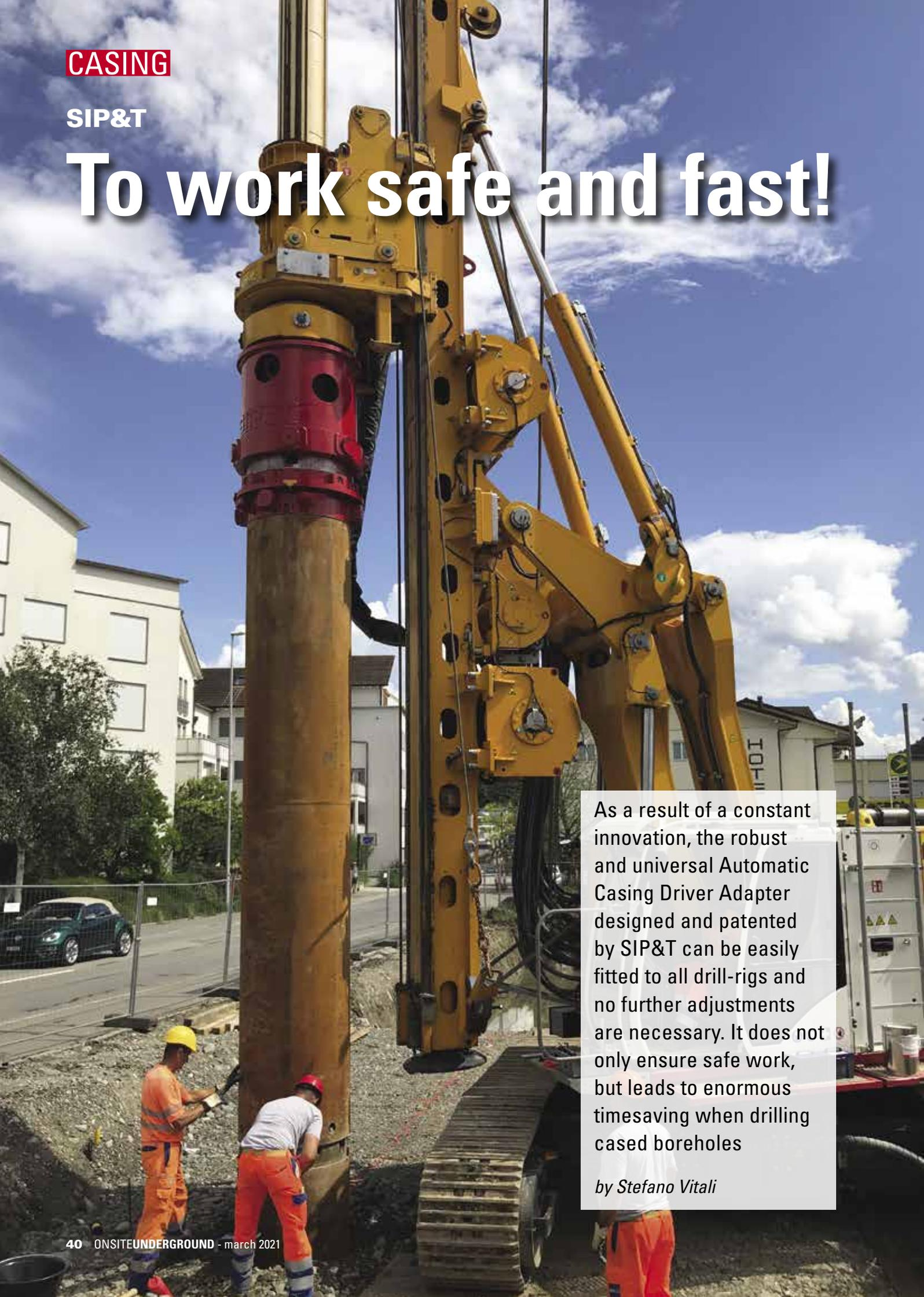
As a result of a constant innovation, the robust and universal Automatic Casing Driver Adapter designed and patented by SIP&T can be easily fitted to all drill-rigs and no further adjustments are necessary. It does not only ensure safe work, but leads to enormous timesaving when drilling cased boreholes
