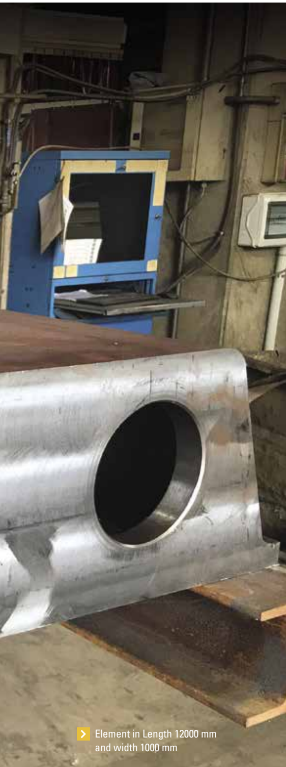
> Trapezoidal shape with rubber seal (water stop) groove and clamshell grab guide channel
